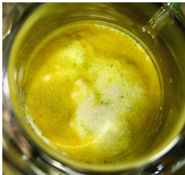
Fig. 2. U crystal in the crystallization experiment (Run6) (after washing).
